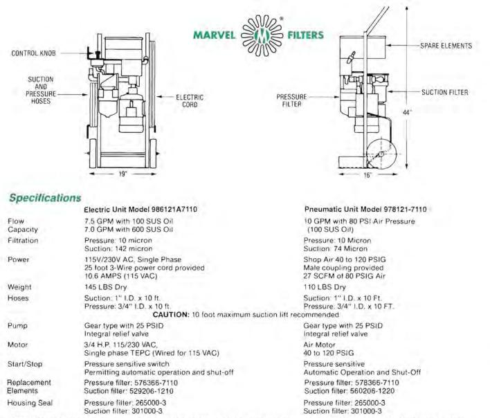
NOTE: Finer and coarser elements available-also elements for use with water glycol and PHOSPHATE ESTER Fluids-consult factory.
