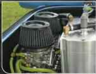
FLAME ARRESTOR #S9-2046 INSTALLED
