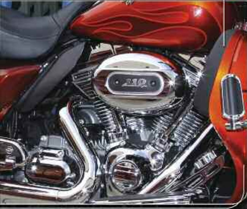
RK Series Intake System Installed
