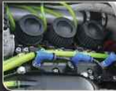
FLAME ARRESTOR #S9-2045 INSTALLED
