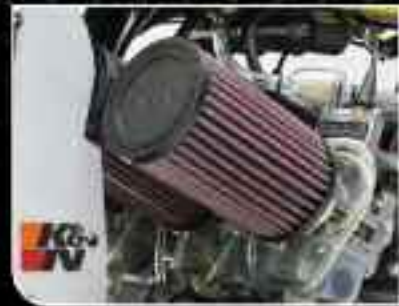
SPECIALTY CLAMP-ON AIR FILTERS INSTALLED
