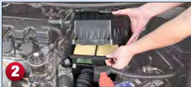
Step 2: Remove the disposable filter.
