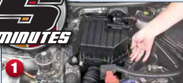
Step 1: Open the vehicle's air box.
