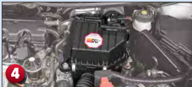
Step 4: Close the air box and apply the "Do Not Discard" decal.
