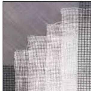
Filter media is shown before K&N® filter oil is applied.
