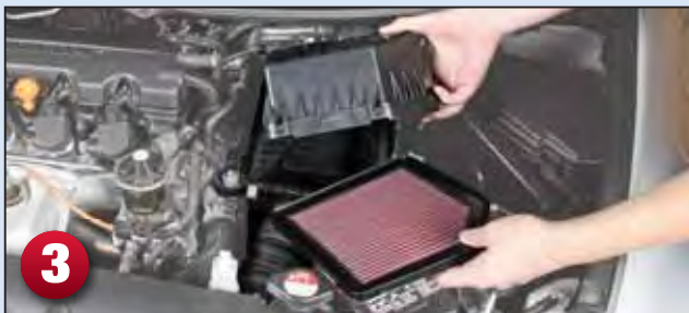
Step 3: Place the K&N Washable/Reusable Air Filter into the air box.
