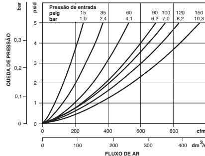
**Teste de queda de pressão de 2 pol.**
