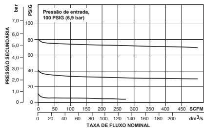
**Teste de queda de pressão de 1-1/4 pol.**
