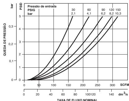
**Teste de queda de pressão de 1-1/4 pol.**
