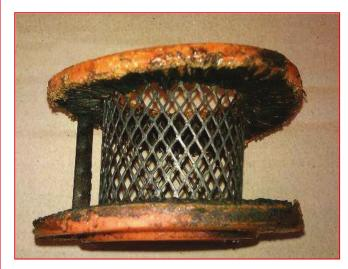
Breather filter burned as a result of explosion in the tank
