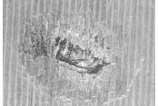
Surface fatigue on ball bearing
