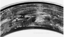
Adhesion on ball bearing
