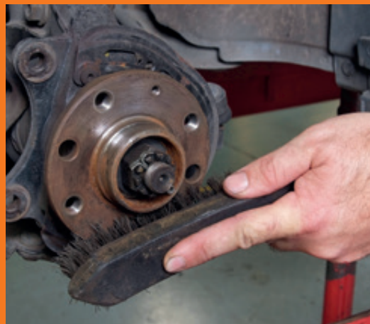
Use a wire scrubbing brush to remove stubborn grime build-up once loosened by the brake cleaner
