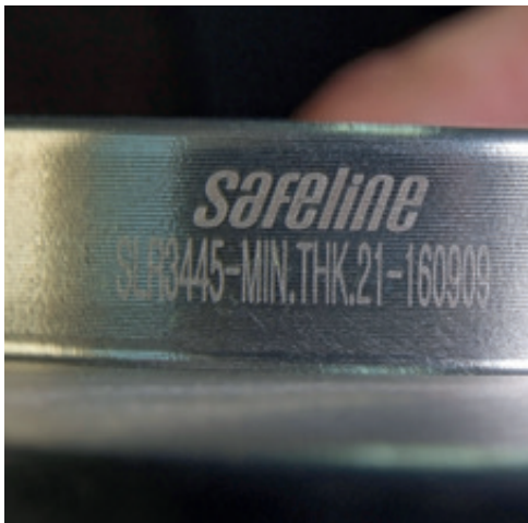
An example of a brake disc thickness specification
