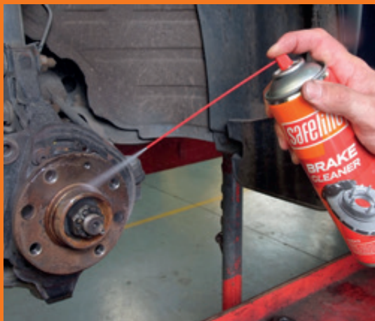
Spray Safeline brake cleaner generously onto the hub to loosen and remove grime build-up
