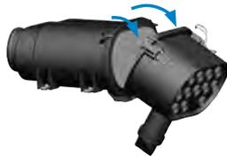
**1 Shut off engine. Unlatch and remove the housing service cover.**
