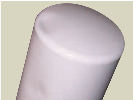
Dents in a steel filter canister create a concentration of stress, making the canister more susceptible to fatigue.
